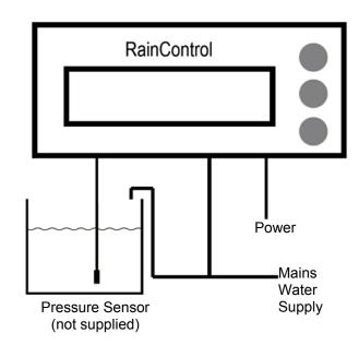
All of the thresholds for high and low water levels can be set by the installer, calibrating the unit to whatever installation the unit is connected to.
